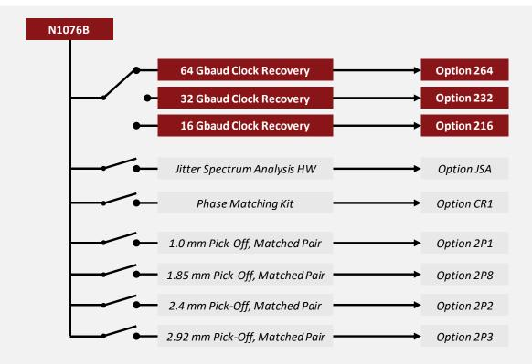
The pick-offs have 2.92 mm connectors on the clock recovery port. The other two ports are male and female with connector sizes as shown above.
