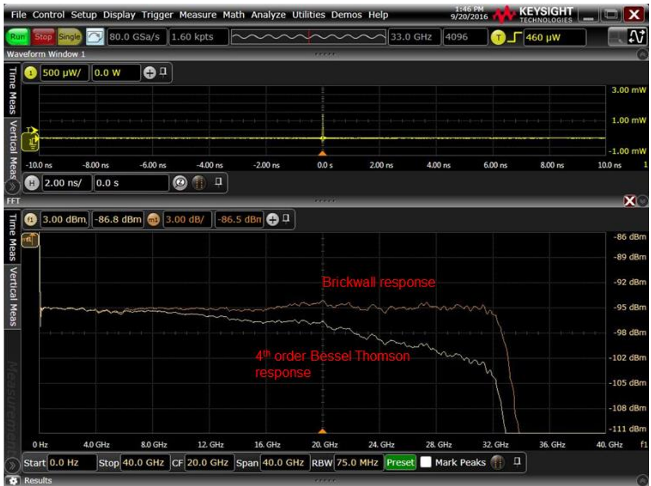
Figure 4. The N7004A used with an Infiniium real-time oscilloscope offers user-selectable hardware Brickwall filter and 4th order Bessel Thomson filter, making the system ideal for reference receiver testing of industry standards or characterizing raw response of optical transmitters.
