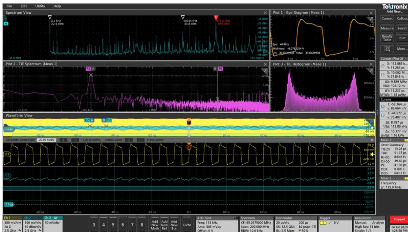
Figure 8: (a) Power rail ripple spectrum and (b) TIE/jitter spectrum.
