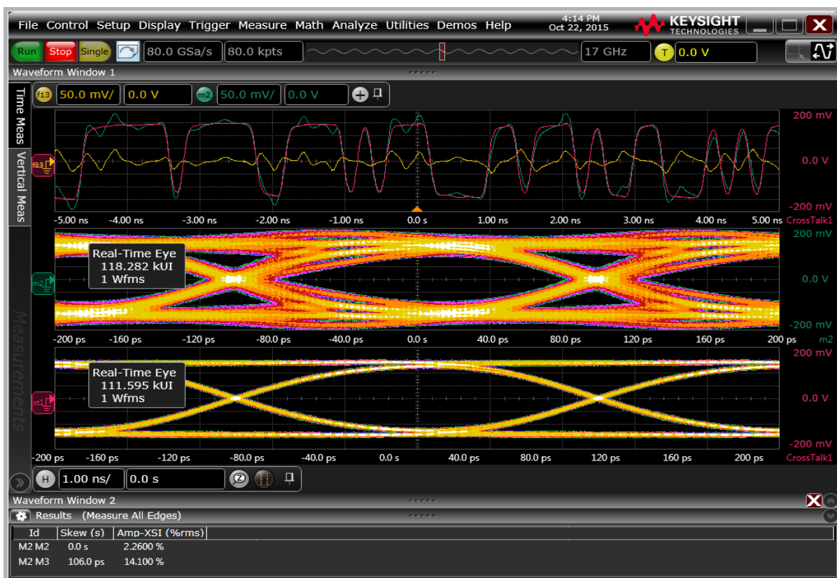
Figure 10. Before and after view of a victim waveform with FEXT. The top plot shows the victim waveform in green, the aggressor in orange, and the crosstalk removed waveform in red. The middle plot is the eye diagram of the victim with the bulging indicative of FEXT, and the bottom plot is the eye diagram of the victim after removing crosstalk.
