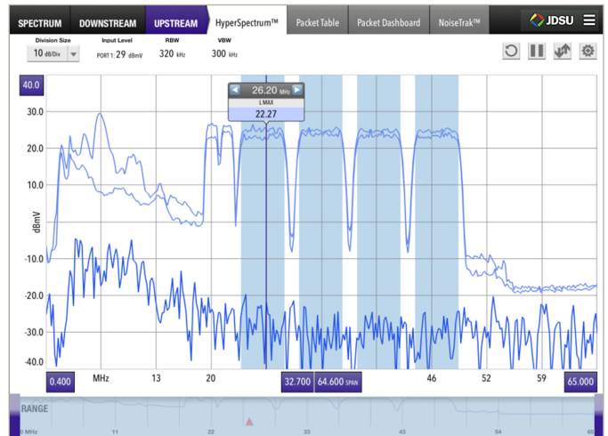
Hyper-Spectrum with upstreams screen
