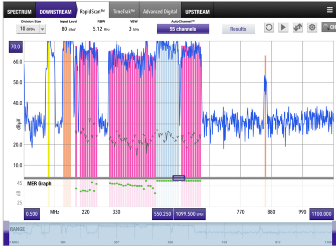
Full downstream channel scan screen
