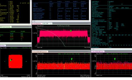
Use 89600 PathWave VSA software to gain deeper insights of DOCSIS 3.1 downstream signals through MER/BER summaries, PLC decoding information, and peak MER traces on the constellation, subcarrier and symbol domains.
