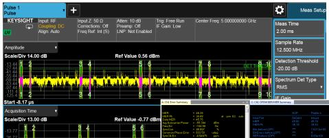
Perform pulse measurements and obtain complete results including power, time, frequency, phase and modulation with the PathWave X-Series Application.
