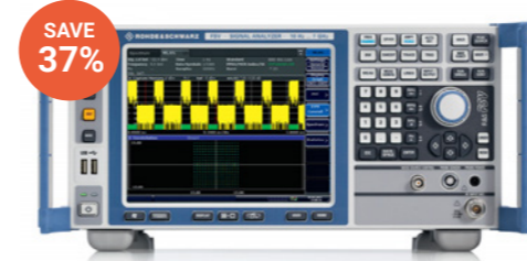
Rohde & Schwarz Spectrum Analyzers-Performance FSV7 (1321.3008.07) Signal and spectrum analyzer 10Hz to 7GHz, -154dBm to +30dBm, resolutionbandwidth 1Hz to 10MHz BUY USED FROM: £20,095 € 22,584
