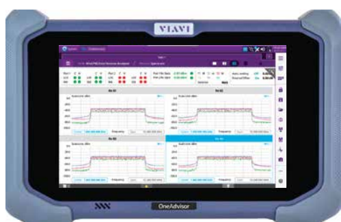
VIAVI OneAdvisor-800 Cell Site Installation Tool
