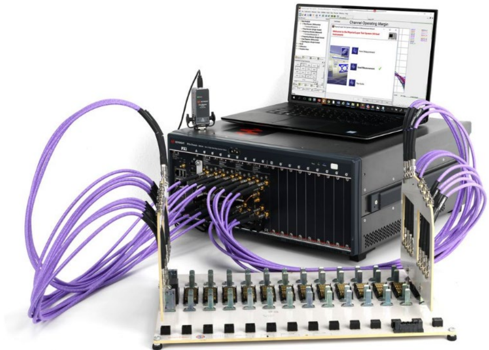
M980xA PXI VNA meets the most demanding multiport challenges with a true multiport architecture.
