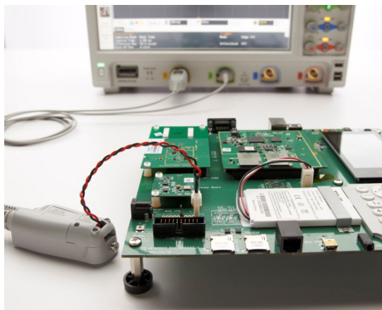
N2820A high-sensitivity 2-channel current probe
