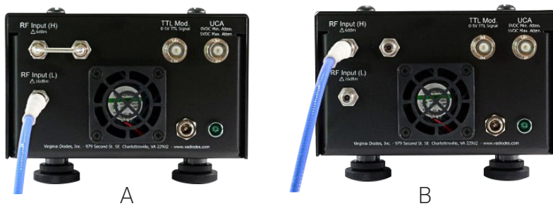
Figure 2. The standard frequency [A] and high frequency [B] RF input modes are shown above. The coaxial jumper connection must be used when using standard frequency operation. With the jumper removed, only the high frequency RF input port is operational.
