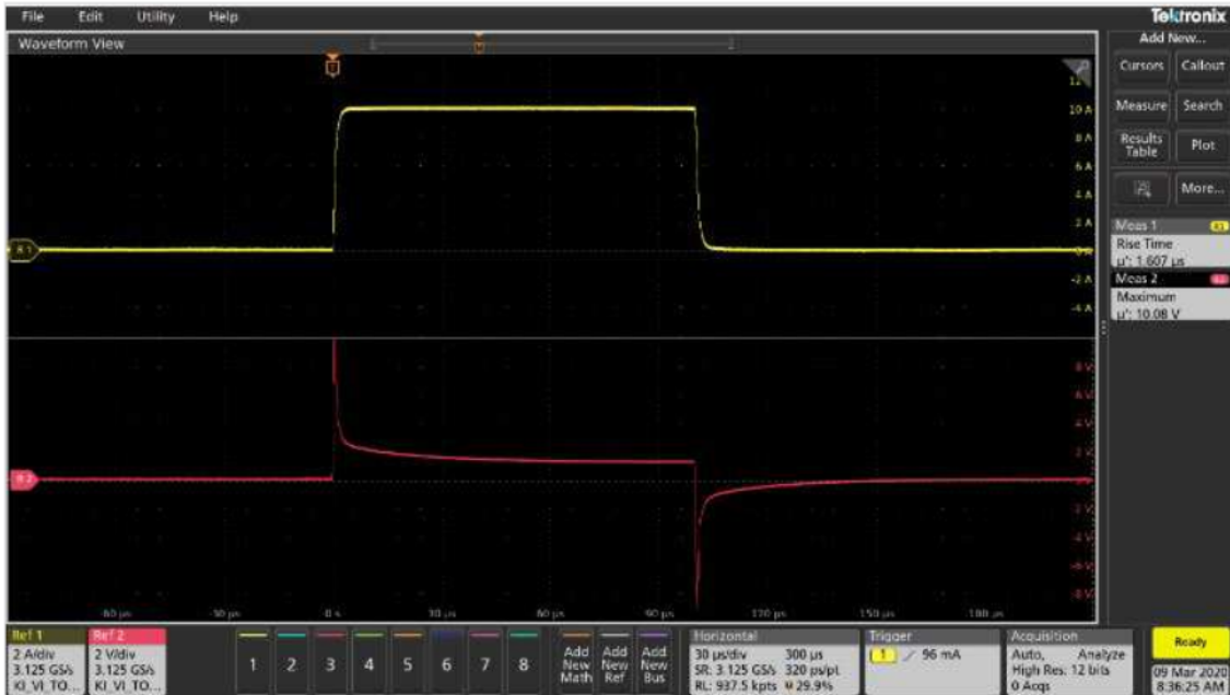
Figure 6. 1.6 \mu\text{s} rise time 10 A pulse on inductor 1 \mu\text{H} .
