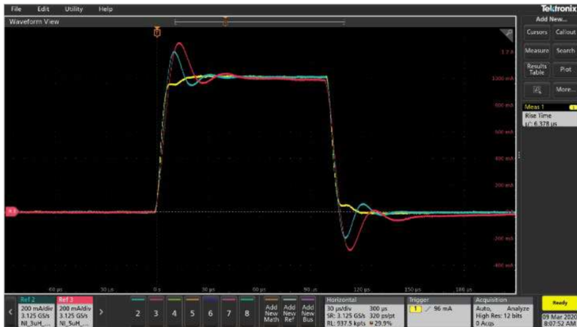
Figure 4. 1 A 100 \mu s pulses on inductors 1 \mu H (yellow) 3 \mu H (blue) 5 \mu H (red).
