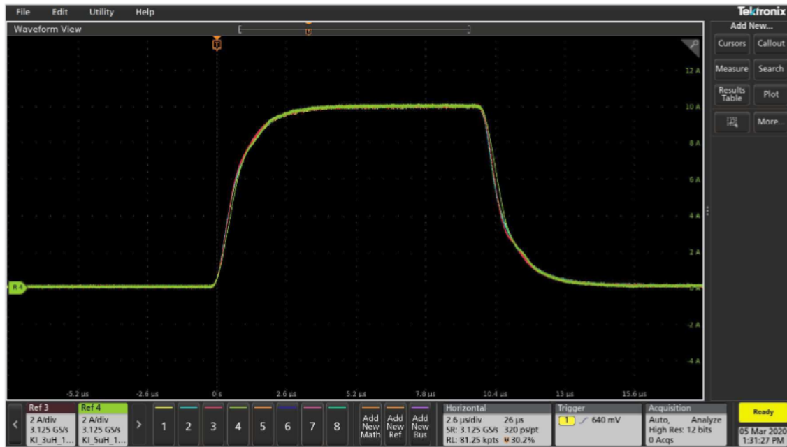
Figure 13. 2601B-PULSE 10 A pulse on 0 \mu H, 1 \mu H, 3 \mu H, and 5 \mu H inductors.
