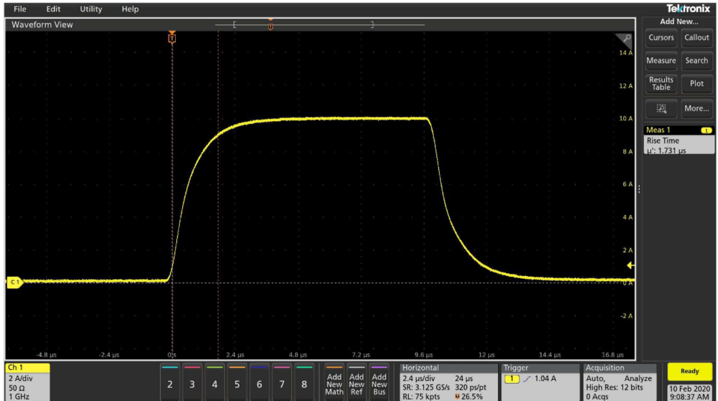
Figure 2: Example of a clean current pulse required for VCSEL testing
