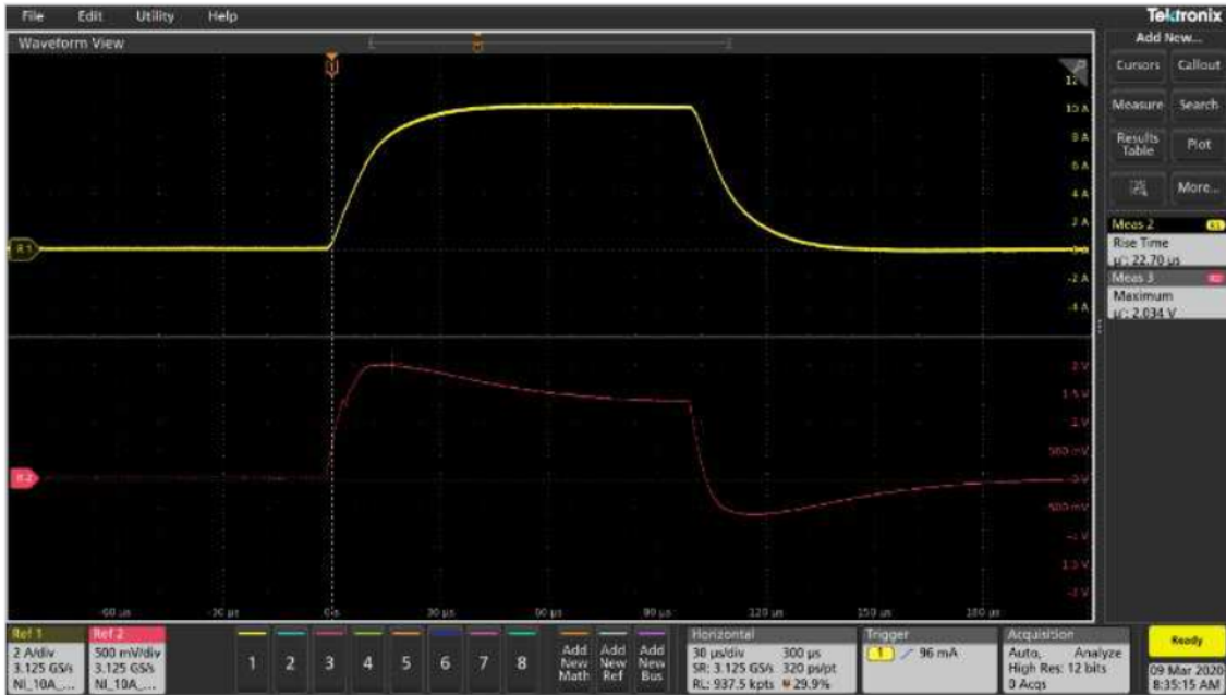
Figure 5. 22 \mu\text{s} rise time 10 A pulse on inductor 1 \mu\text{H} .
