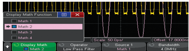
Figure 32. Four math functions can be created and nested with one resultant math function.
