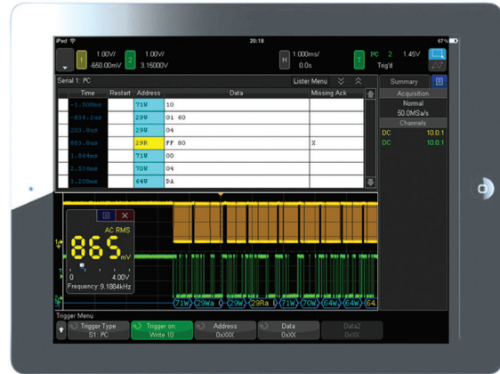
Figure 38. Tablet virtual front panel control.
