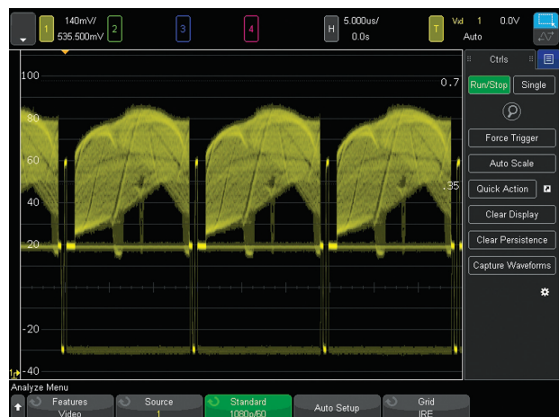
Figure 27. Triggering on 1080p HDTV signal analysis.
