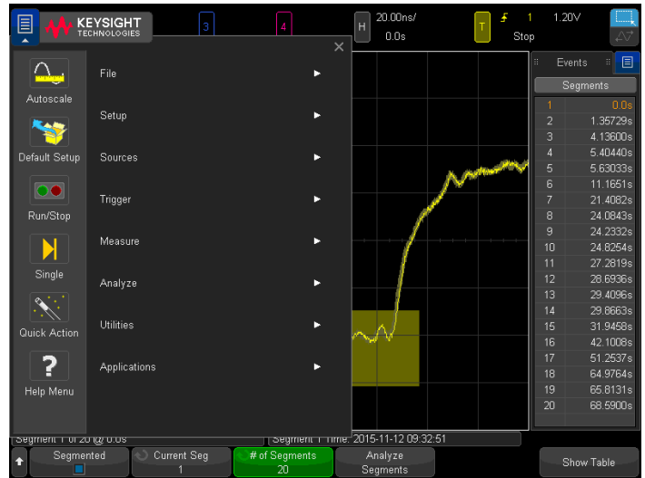
Figure 14. Use the Keysight pull-down menu for Windows-like operation.
