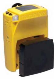
Nardalert S3 Mainframe shown with interchangeable sensor.
