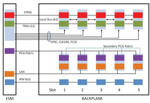
Figure 2. M9505A backplane block diagram
