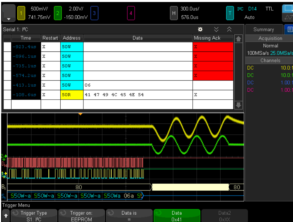
Figure 1. Decoding and triggering on an I 2 C bus using a Keysight mixed signal oscilloscope (MSO) licensed with the Embedded Software Package.
