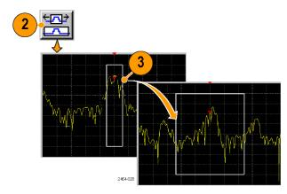
You can also tap the Region Span field in the Region drawer to enter a specific frequency span for the region.
