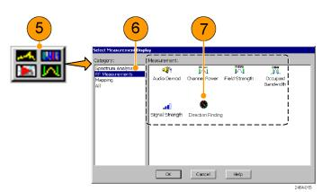
8. Enter values in the RF Measure drawer, Signal Strength and Settings tabs, and other instrument control fields to set the measurement parameters. Tap the help [?] button in the RF Measure drawer or on the measurement tabs for help on those fields.
