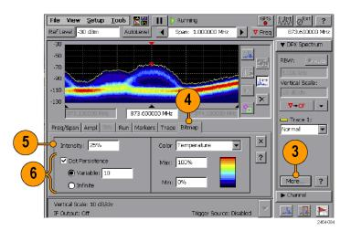
Tap the Dot Persistence check box to enable Bitmap point display persistence controls. Dot persistence sets how long a point is displayed if it is not updated with new data.
