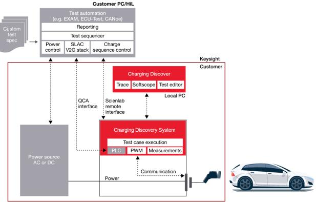
Figure 7. Interface topology of CDS with Developer mode.
