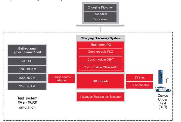
Figure 1. Modularity of the Scienlab Charging Discovery System - Portable Series.
