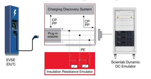
Figure 3. System topology including Scienlab Isolation Resistance Emulator.
