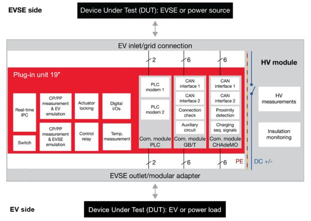
Figure 2. Block diagram of CDS architecture.
