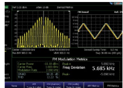
Characterize AM/FM signals using AM/FM demodulation
