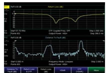
View return loss and DTF simultaneously
