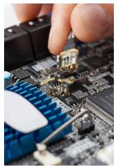
N2848A InfiniiMax III 16 GHz QuickTip head
