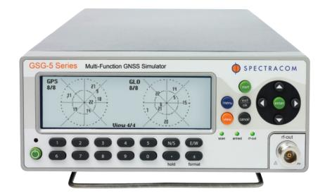
The GSG-56 is the latest offering of the popular GSG-5x family of simulators from Spectracom. In addition to all the features of the advanced GSG-55, it provides simultaneous simulation of the L1 signals of GLONASS and GPS systems as well as all the currently operating Satellite-Based Augmentation Systems [SBAS] for worldwide coverage.
