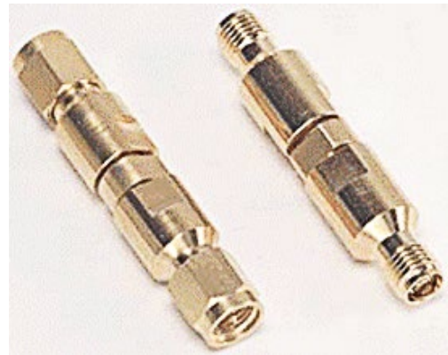
Figure 3. “Connector savers” are coaxial adapters placed between instrument front-panel connectors and cables or DUTs. They can be easily replaced if they are damaged or become worn. Source: Keysight.com
