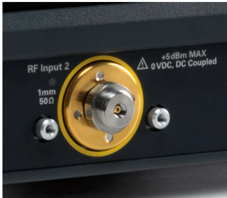
Figure 2. While the typical front-panel connector is female, the gender is often reversed for equipment covering millimeter frequencies (30 GHz to 300 GHz). The male connector offers some degree of protection from several types of damage. Source: Keysight.com
