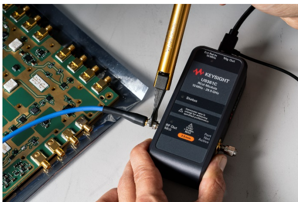
Figure 7. The U9361 Series RCal Receiver Calibrator effectively moves the reference plane to the DUT to improve your test Rx system accuracy by an order of magnitude. Source: Keysight.com
