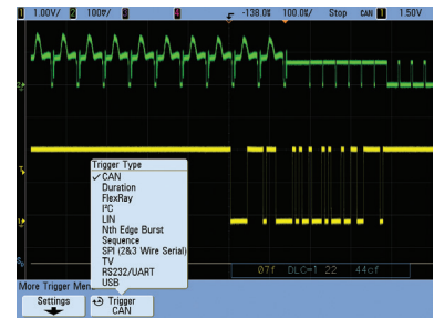
Trigger on and decode CAN serial packets.
