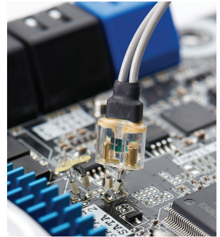
Figure 12. Use InfiniiMax III+ probe amplifier with QuickTip head for quick and secure magnetic connection.
