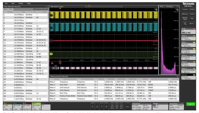
Viewing four analog channels, a decoded serial bus waveform, decoded serial packet results table, seven measurements, a measurement histogram, measurements results table with statistics, and a DVM - simultaneously!
