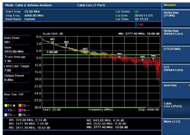
Cable and antenna test — Cable Loss
