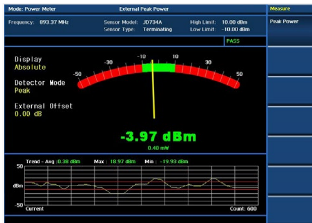
Power meter test (RF or optical)
