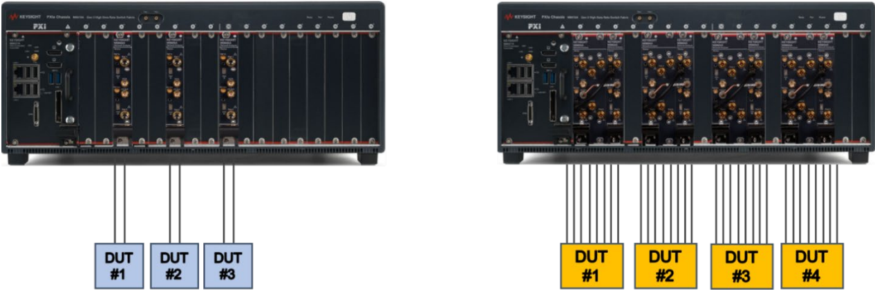
Examples of multi-site measurement configurations
