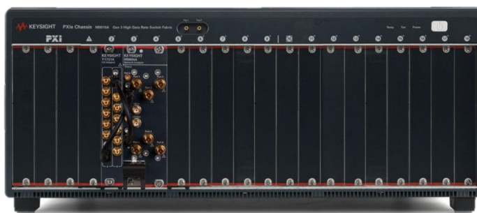
Connecting M9804A (right) and Y1731A option 001 (left) for coaxial interfaces
