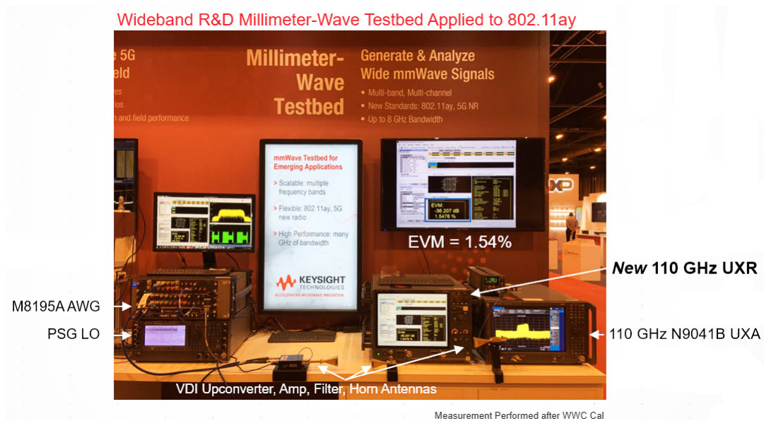
Figure 4: Millimeter-wave R&D testbed with the 110 GHz ultra-high performance UXR oscilloscope
