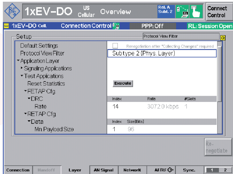
The structure of the 1xEV-DO protocol stack is mapped onto an advanced menu structure for use by R&D and production engineers.
