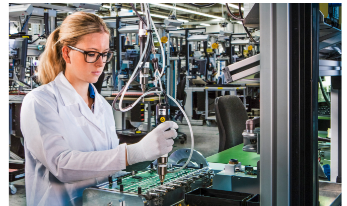
Manual component placement at the Rohde & Schwarz Memmingen plant, Germany.
