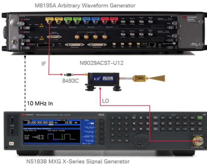
Figure 4. Receiver verification instrument setup
