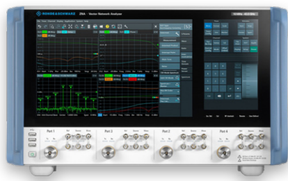
Rohde & Schwarz ZNA43 | Vector Network Analyzer; 4 ports, 10 MHz to 43.5 GHz
