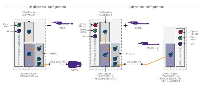
The innovative VIAVI multi-test access unit connection schematic showing the relevant link characterization test functions
