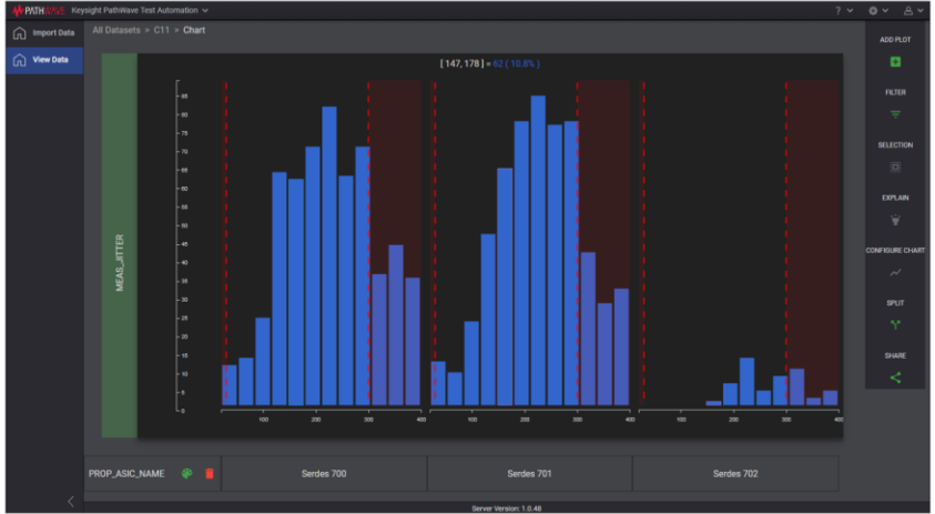
Figure 5: User can import test results to the KS6810A software from the DDR5 Tx Compliance Test software and view the test results with the visualization tool.
