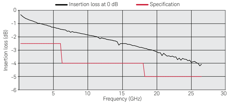
Figure 4. Keysight J7211A attenuation control unit insertion loss (at 0 dB) versus frequency
