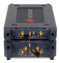
4-port configuration using two P937xA VNAs (left), 6-port configuration using 2-port P500xA and 4-port P502xA (right).
