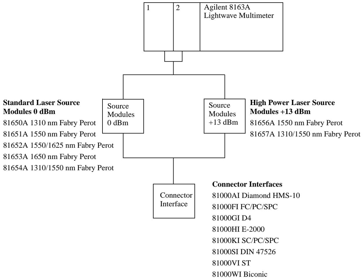
**Figure 5 Recommended Connector Interfaces**
