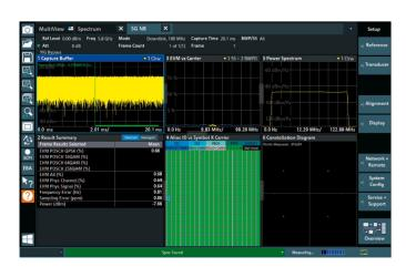
Analysis of a 5G NR signal with the R&S®FSV3-K144 (downlink) and R&S®FSV3-K145 (uplink) options
