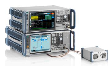
R&S®FExxDTR external frontend with R&S®SMM100A vector signal generator and R&S®FSVA3000 signal and spectrum analyzer.
