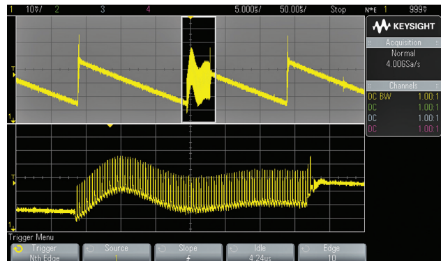
4M deep memory captured a long time span without losing the details.
