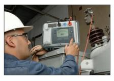
Circuit breaker being tested with the S1-552 Insulation Resistance Tester
