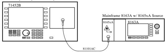
Figure 6 Measurement Setup for Center Wavelength and Spectral Bandwidth
