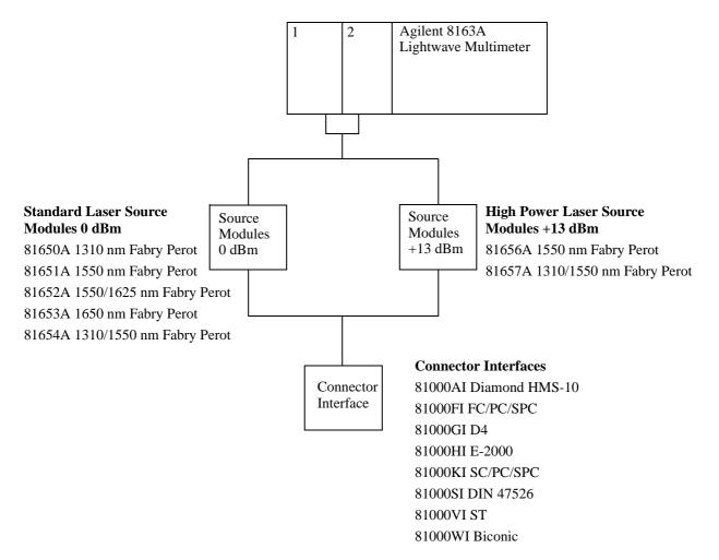
Figure 5 Recommended Connector Interfaces
