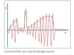
In both operating modes CC and CR, the ZSAC load can simulate load profiles with the LIST function. Up to 50 setpoints of variable duration with associated ramp time are possible. In AC mode, the LIST function serves as an envelope of the effective value.
