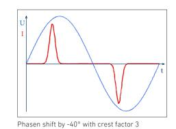
By programming a crest factor (0 ... 10), the ratio of peak value to rms value of the load current is changed in such a way that the sine half-waves are compressed in terms of time.
