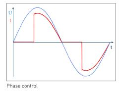
A phase cut angle can be programmed for each half-wave, which is set to 0 during execution. The two angles can be defined independently of each other from 0 to 180°. For example, an entire half-wave can be deleted.
