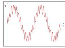
The scaled amplitudes of the odd-numbered harmonics, i.e. 1st to 15th harmonics, are defined with 8 parameters.
