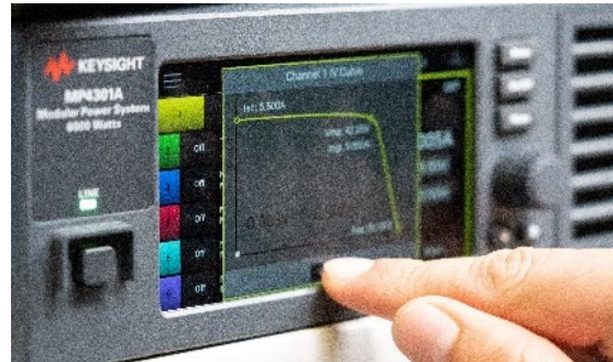
Figure 4. Intuitive touch display, setting SAS curve
