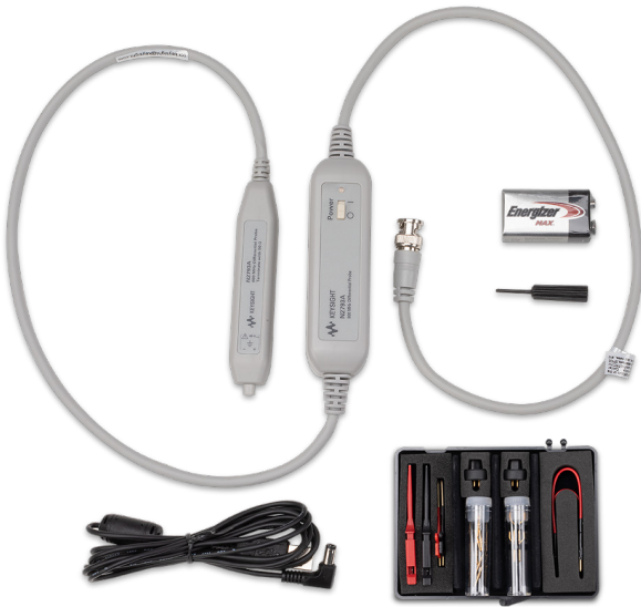
Figure 8. N2793A 800 MHz differential probe with standard accessories
