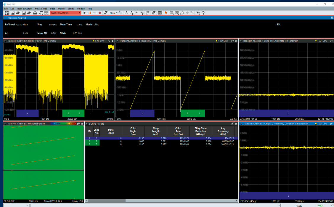
Fig. 4: Transient analysis of a chirp sequence signal with the R&S®VSE-K60C transient chirp measurements option. The pulse power versus time is shown at the top left. The linear frequency response can be seen in the top middle and in the spectrogram on the bottom left. The software lists the properties of the detected pulses in a table (bottom middle). The properties can also be investigated in detail in graphical form. The chirp rate and frequency deviation are shown on the right.
