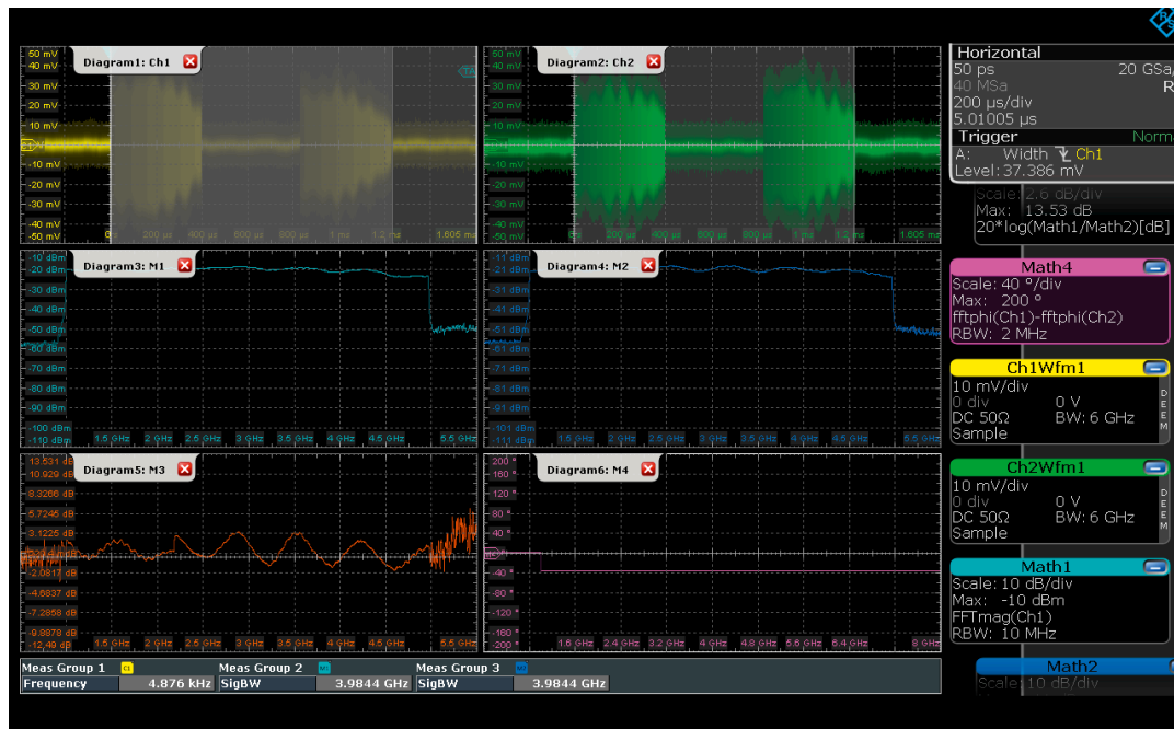
Fig. 5: Multichannel measurement of a chirp sequence. The pulses are shown in the time domain (top), the spectra of the individual channels in the middle, and the amplitudes and phase difference are shown on the bottom left and bottom right, respectively.
