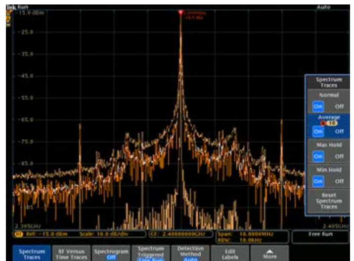
Figure 17: Normal, Average, Max Hold, and Min Hold spectrum traces
