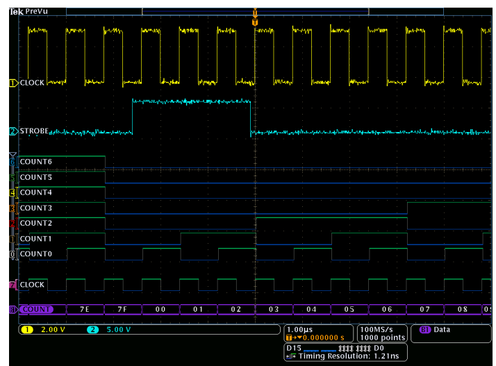
Figure 29: The MDO4000C Series provides 16 integrated digital channels enabling you to view and analyze time-correlated analog and digital signals.
