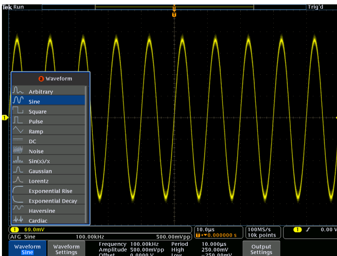
Figure 27: Waveform type selection in the integrated AFG.
