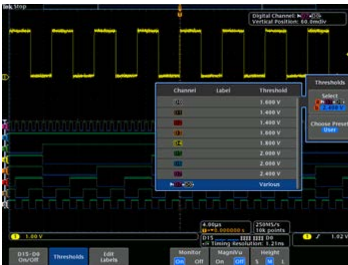
Figure 30: With color-coded digital waveform display, groups are created by simply placing digital channels together on the screen, allowing digital channels to be moved as a group.
