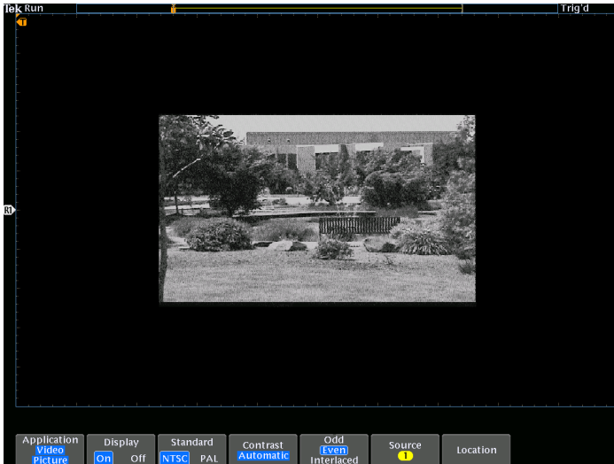
Figure 10: Viewing an NTSC video signal. Video picture mode contains automatic contrast and brightness settings as well as manual controls.
