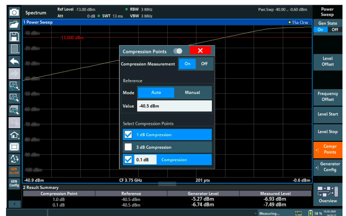
Measurement of 1 dB and 0.1 dB compression points
