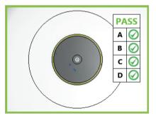
User-Definable Pass/Fail Acceptance Criteria Whether using the IEC 61300-3-35 or customer-specific requirements, users can easily manage user-specified acceptance criteria with dedicated profiles for each requirement.
