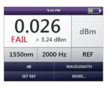
Accurate Measurement and Simple Operation Make quick, easy dual-wavelength measurements at 850 and 1300 nm or 1310 and 1550 nm using saved reference levels.
