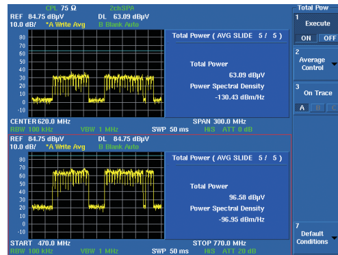
Simultaneous measurement of input/output for feed-forward amp
