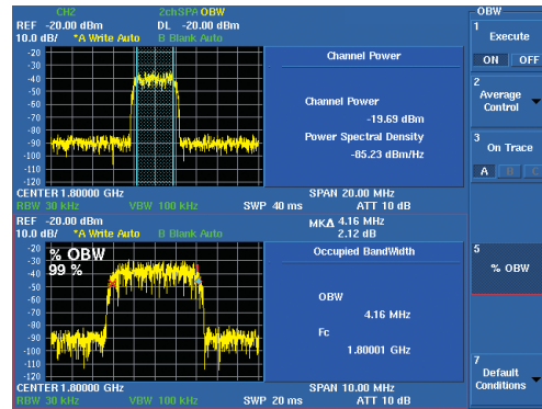
Simultaneous measurement of POWER and OBW
