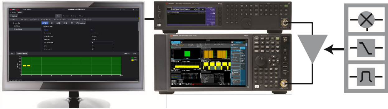
Figure 2. Typical component test configuration using PWSG desktop with an X-Series signal generator and analyzer.
